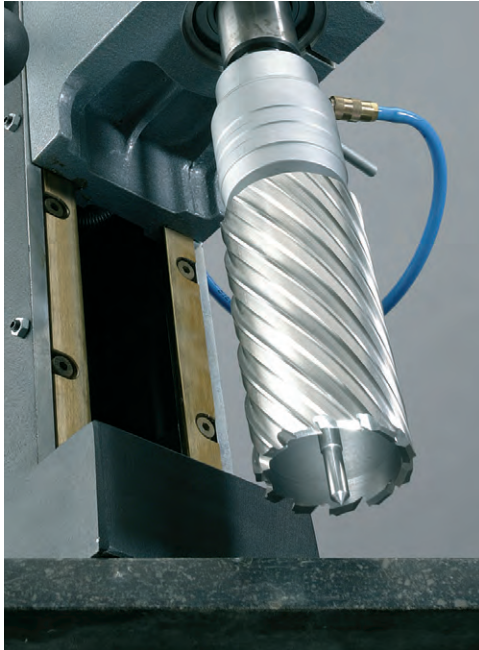
Annular Cutter Recommended Revolutions Per Minute Recommended Feed Rate: .002 - .004 inches per revolution
